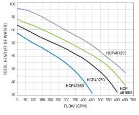
All motors: Certified to UL 1004, IP 55 protection, insulation class F. 60 hz.,  $3.550 \ \text{RPM}$
