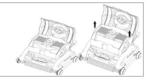
Flip the bucket assembly over to remove the debris & then rinse with a garden hose to remove small particles. <u>Filter cartridges do not need to be</u> <u>removed to clean.</u>
