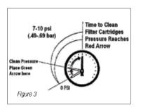
pressure reading, line up the green arrow with the current reading, (See Fig 3) When the pressure rises to or above the red or second arrow, it is time to clean or replace your filter cartridge elements.
